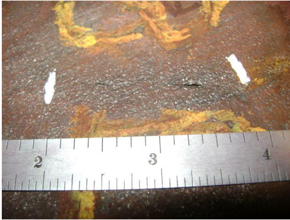
Figure D.26. Indication 1 at gage 8 (after 2 million cycles)
