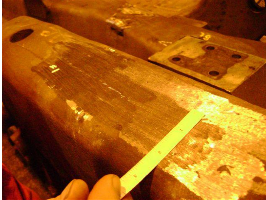
Figure D.36. Indication 1 at gage 8 (top of pedestal after 6 million cycles and grinding)
