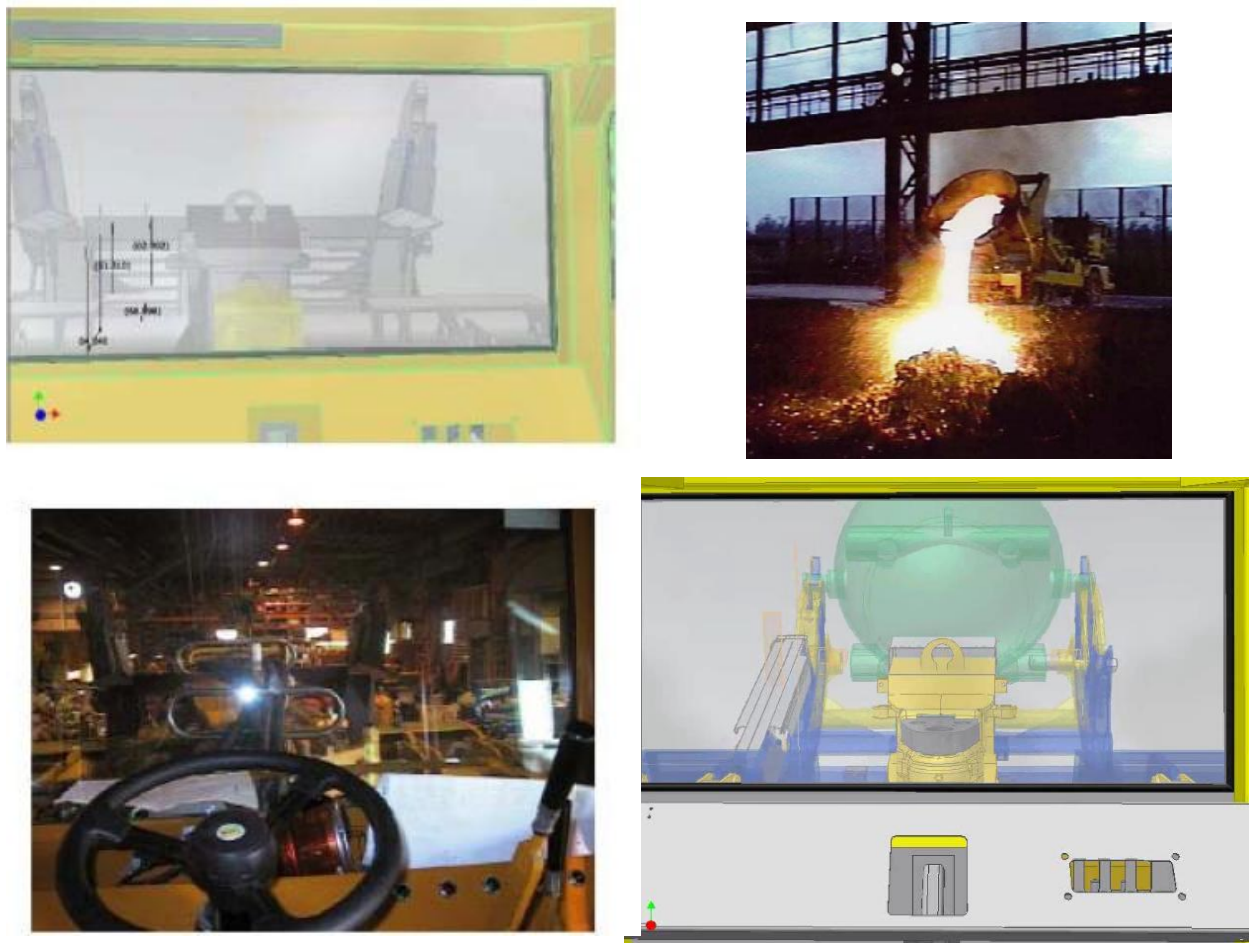
Figure 3.7. Crucible being rotated in kinematic study and synthesis in 3 point perspective through high fidelity CAD environment – a unique approach to kinematic synthesis problem.
