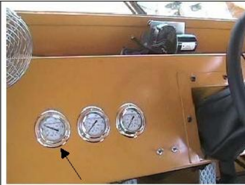
Highest reading on the Bourdon gage as the test weight is lifted at 1650 psi
