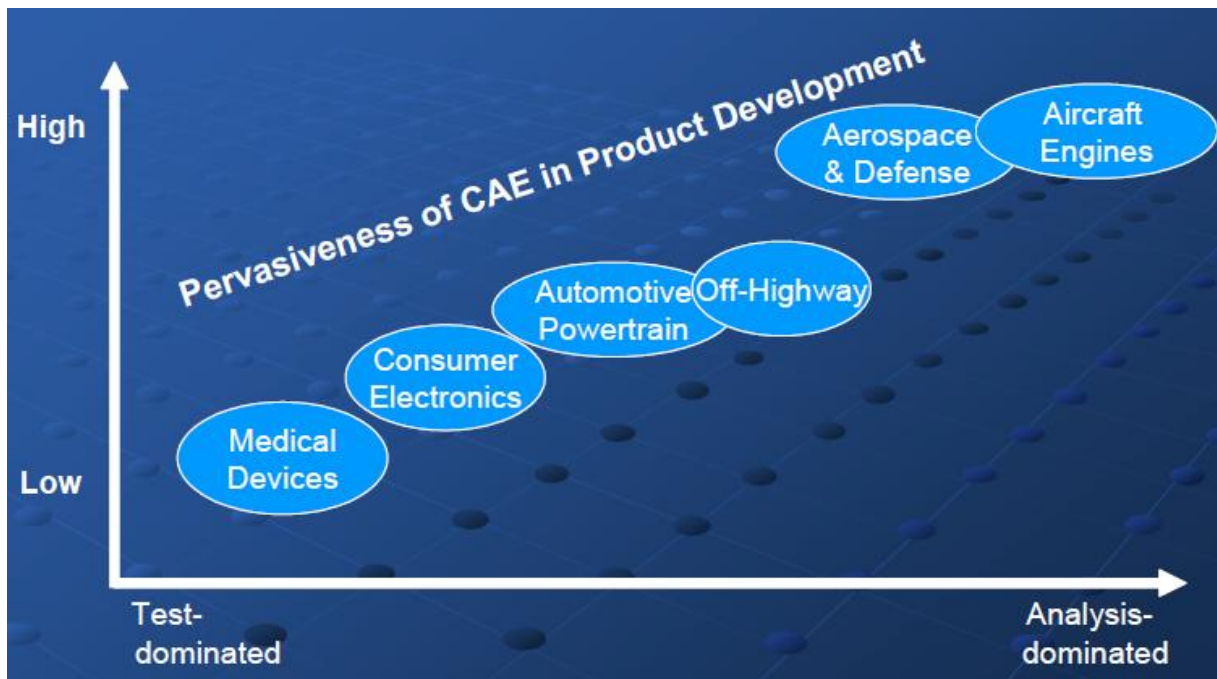
Figure 1.3. Usage of CAE in various industries. CAE for the category of ground vehicle engineering (automotive power train and off-highway) is seen to still have untapped potential to play greater role over physical prototype/test as compared to aerospace engineering (59).
