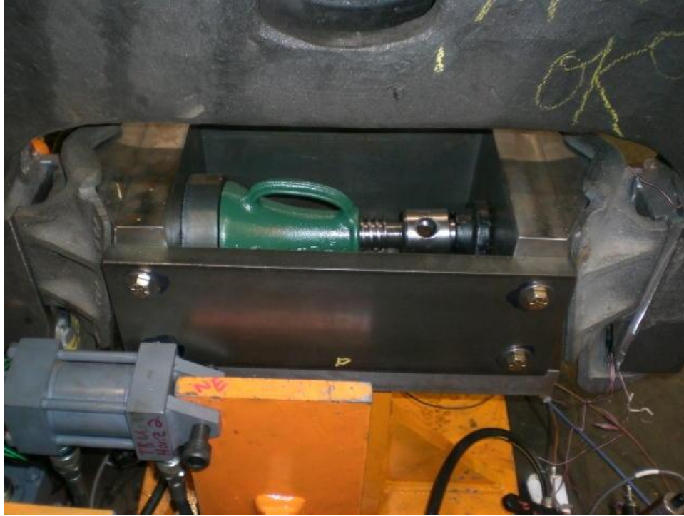
Figure D.16. Machined Pedestal Supports
