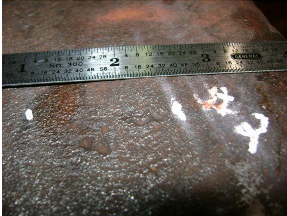
Figure D.32. Indication 2 (after 4 million cycles)
