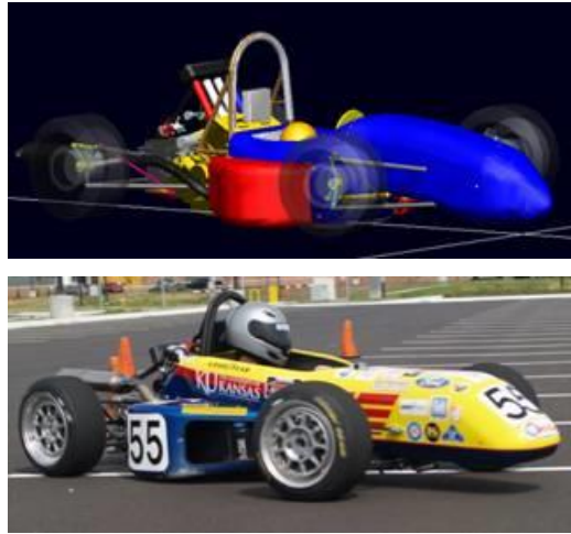
Figure 2.4. Virtual prototype of University of Kansas Formula SAE car - full vehicle simulation is faster than real time.
