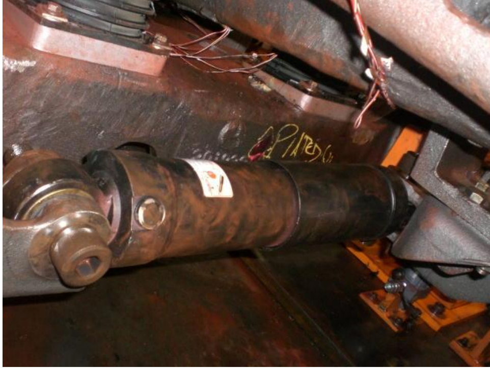
Figure D.22. Longitudinal Damper and wired strain gages.
