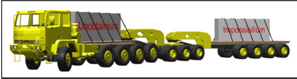
Figure 1.9. Example of a virtual model, which appears realistic and feasible. The design however, cannot be supported with sound engineering projection beyond the third axle, when factoring in real world strength, performance, size, and weight considerations (21).
