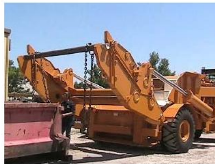
Machine in position for test setup with 2 x 38000 lbs mockup weight.
