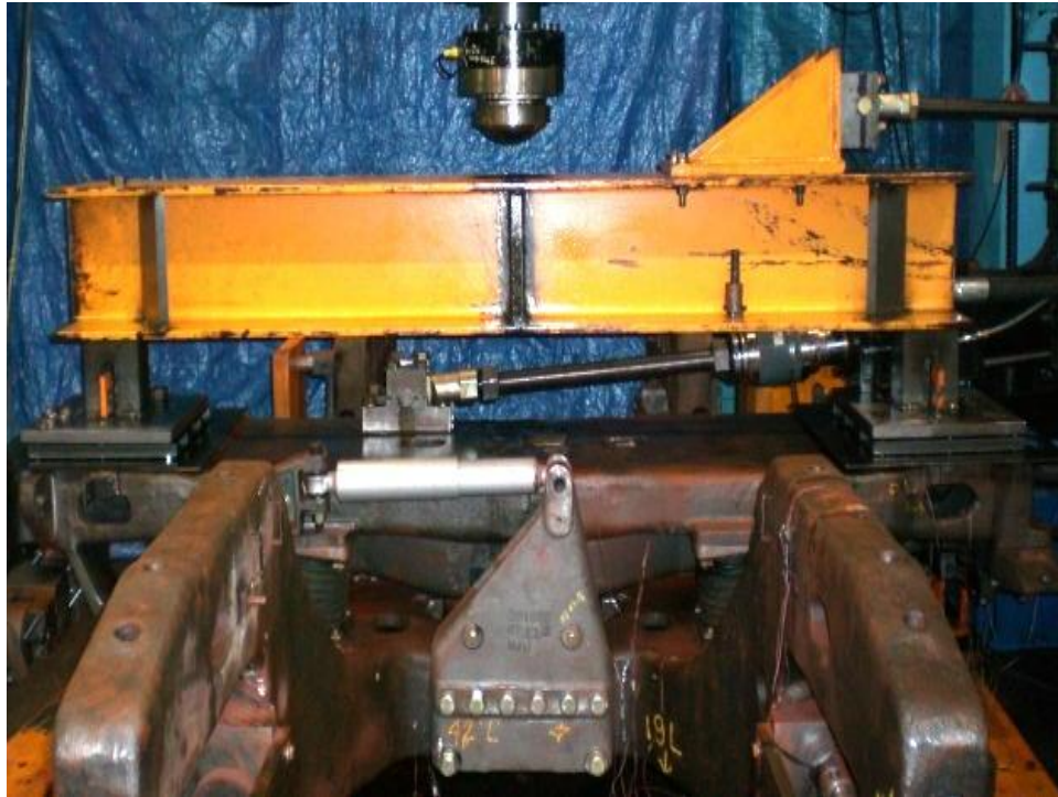
Figure D.17. Application of the Vertical Load
